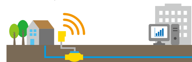
Automatic meter reading and water leak detection
