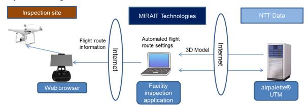
■ Image of automated flight route settings based on a 3D model
