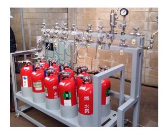
First in Japan to simultaneously fill 10 high-pressure hydrogen containers at 29.4 MPa
